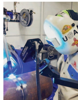
The WeldWatch weld camera is being used here by Welding Instructor Justin Forni as he demonstrates a weld to students over Zoom.
